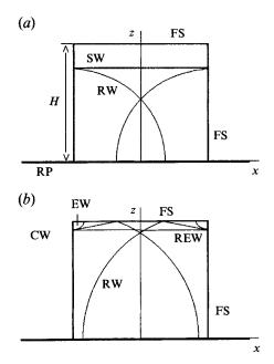
FIGURE 7. Impact by a finite liquid cylinder (a plane case is shown). (a) The wave pattern at the initial stage when the presence of the upper free surface does not affect the flow: FS, free surface; SW, shock wave; RW, relief wave; RP, rigid plate; H, length of the cylinder. (b) Reflection of the shock wave at the upper free surface of the cylinder: REW, reflected expansion wave; EW, edge wave; CW, compression wave.
