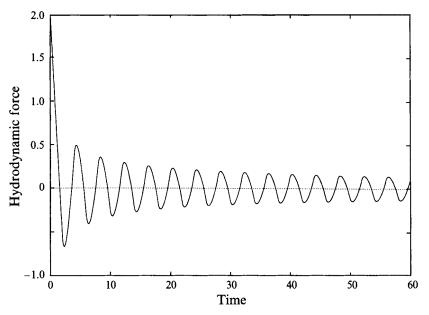
FIGURE 3. Hydrodynamic force F(t) on a plate impacted by a plane jet.
