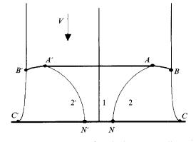
FIGURE 8. The wave pattern at the initial stage of the jet impact (nonlinear theory, plane case): AA', undeformable part of the shock front; AB and A'B', curved parts of the shock; AN and A'N', fronts of the relief waves; BC and B'C', disturbed parts of the jet free surface; V, jet speed. The liquid is at rest in region ANN'A', the flows inside regions ABCN and A'N'C'B' are self-similar at the stage shown.
