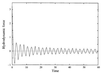
FIGURE 5. Hydrodynamic force F(t) on a plate impacted by an axisymmetrical jet.
