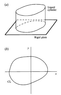
FIGURE 6. Impact of a plate on a liquid cylinder of arbitrary cross-section. (a) General view at the initial moment. (b) The bottom view: CL, contact line between the liquid free surface and the plate.
