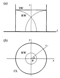
FIGURE 4. Impact of a plate on a liquid circular cylinder. (a) The side view of the wave pattern at the initial stage of the impact (axisymmetric case): SW, shock wave; RW, relief wave; r, radial coordinate. (b) The bottom view: CL, contact line between the liquid free surface and the plate; relief wave, RW, converges to the centre point.
